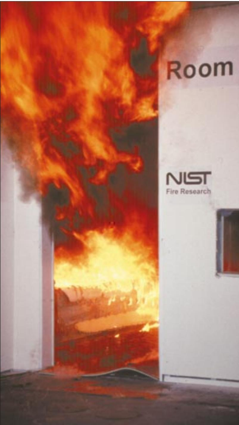
Part of a series of flashover fire tests conducted by NIST.
