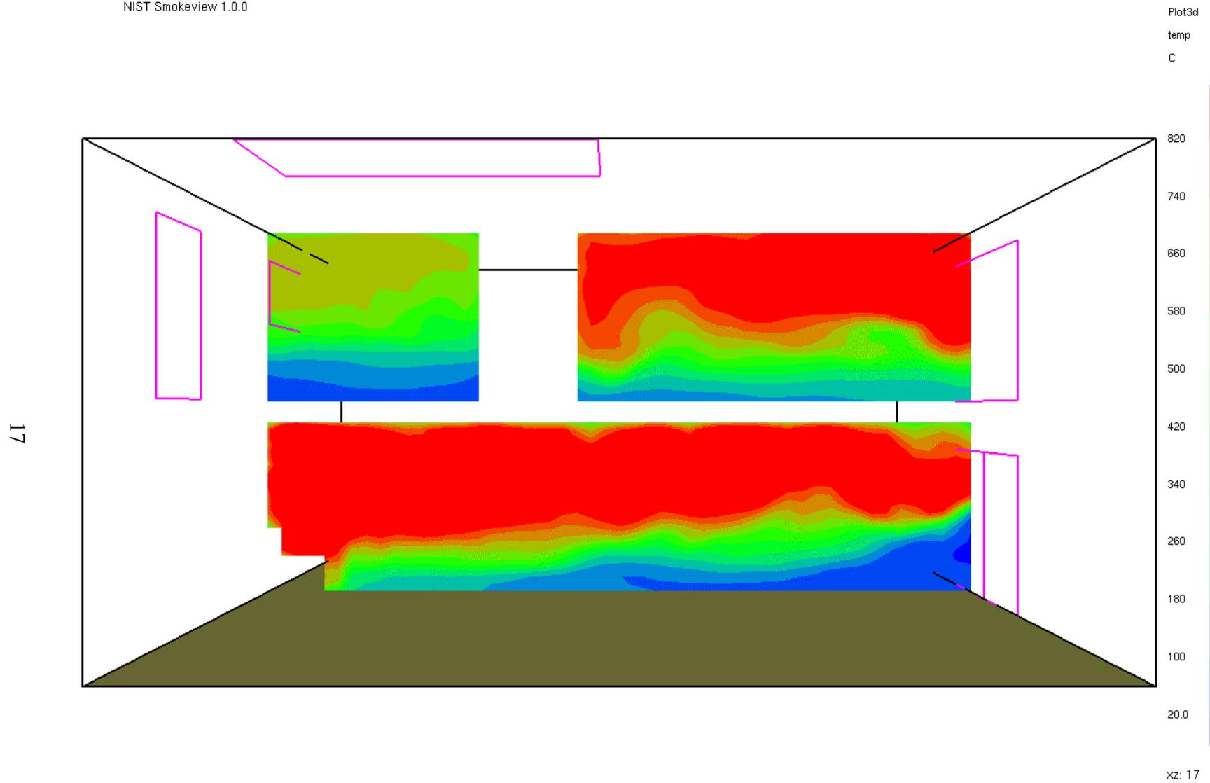
Figure 6. Temperature slice along basement sliding glass door, at 200 seconds of simulation.
