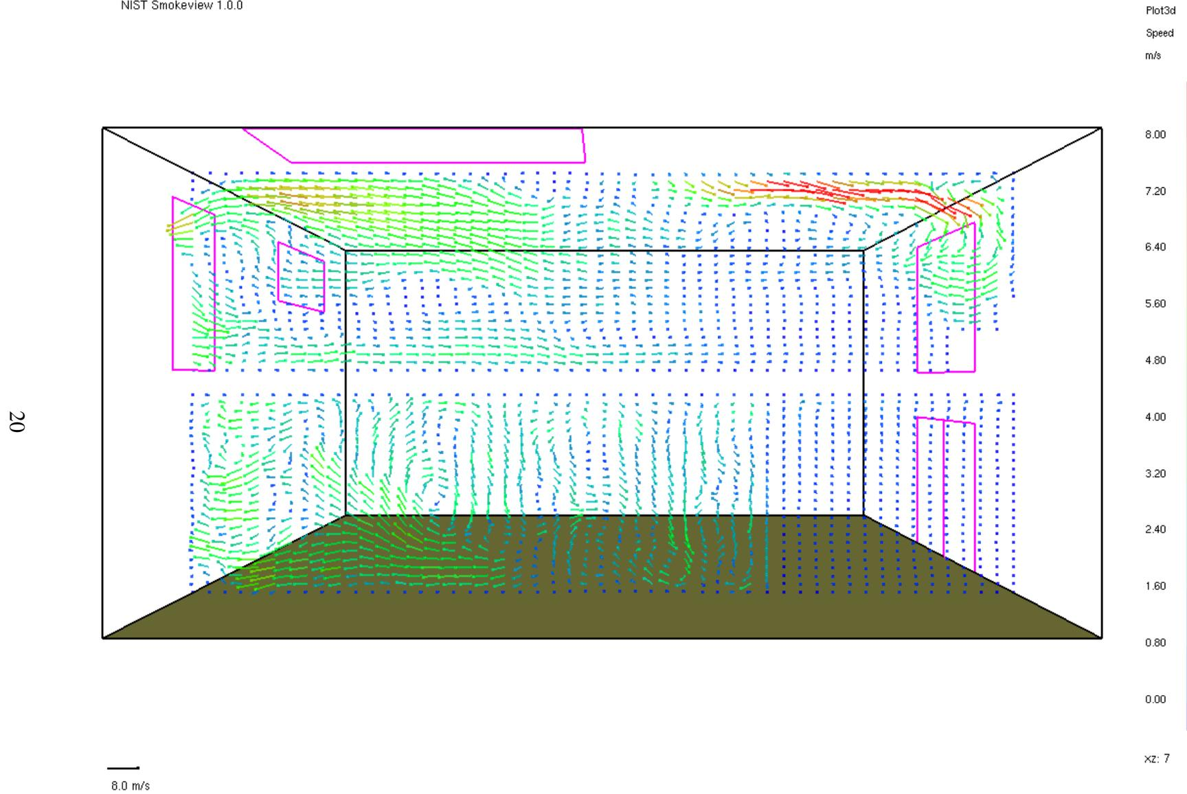
Figure 9. Vector representation of velocity slice along front door, at 200 seconds of simulation.
