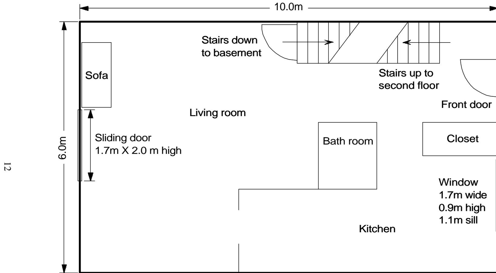
Figure 1. Plan view of first floor.
