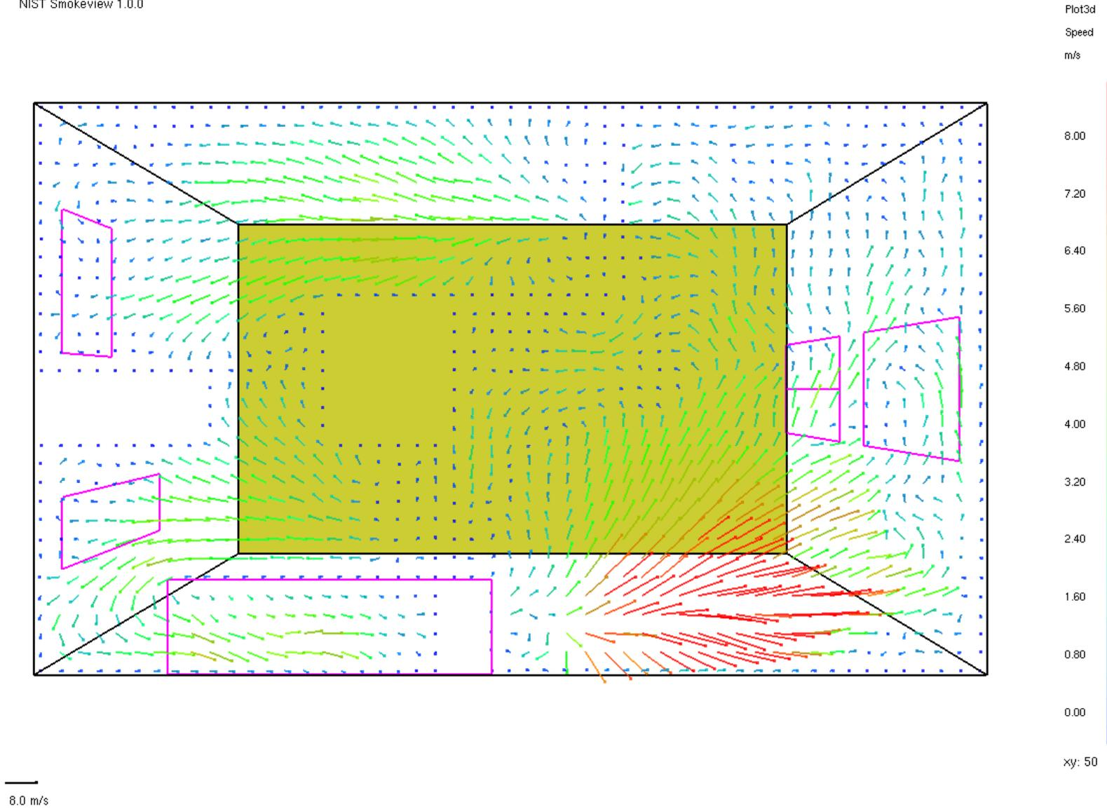
Figure 14. Vector representation of velocity at the ceiling, at 200 seconds of simulation.
