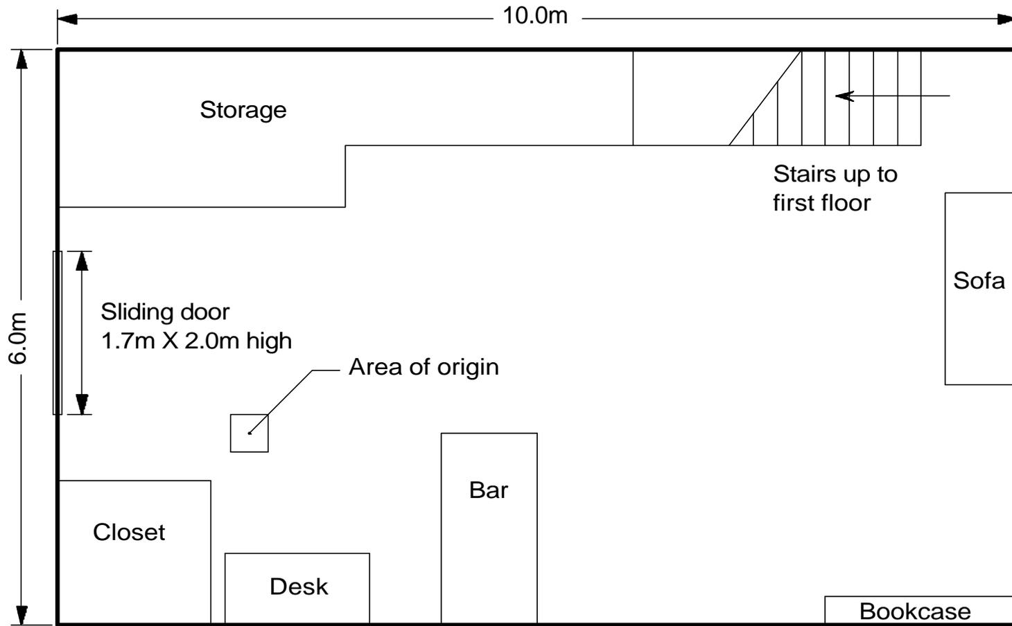
Figure 2. Plan view of basement.
