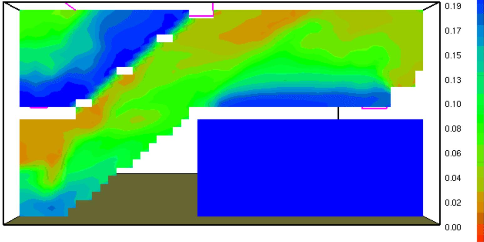
Figure 13. Percent oxygen along centerline of stairway, at 200 seconds of simulation.
