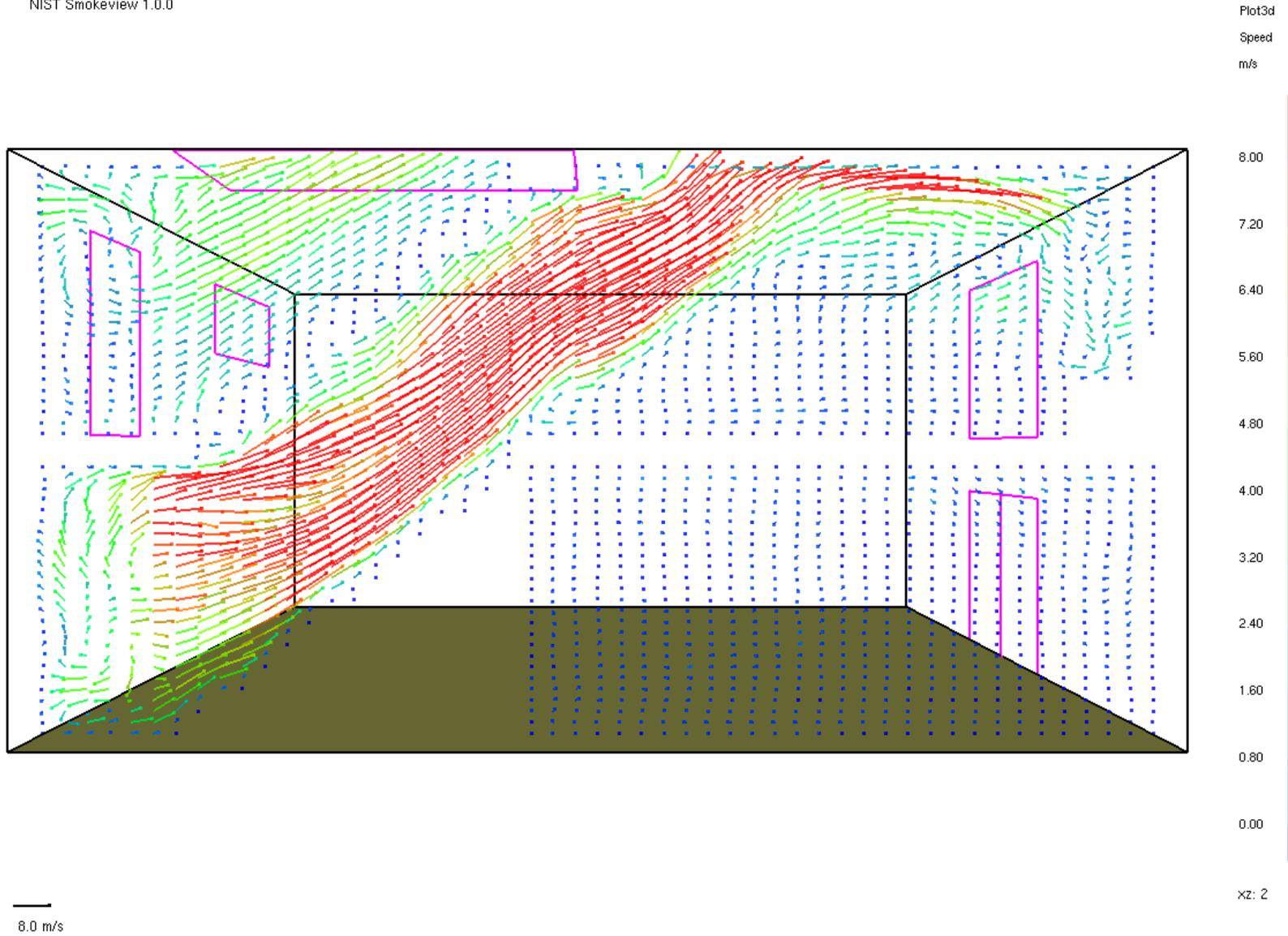
Figure 11. Vector representation of velocity along centerline of stairway, at 200 seconds of simulation.
