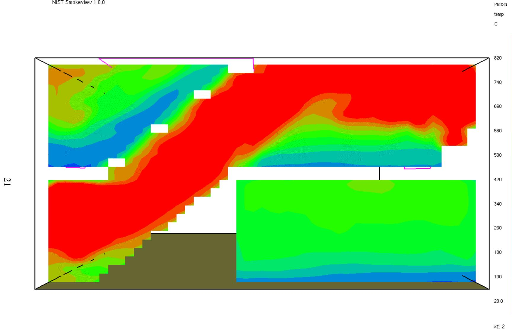
Figure 10. Temperature slice along centerline of stairway, at 200 seconds of simulation.
