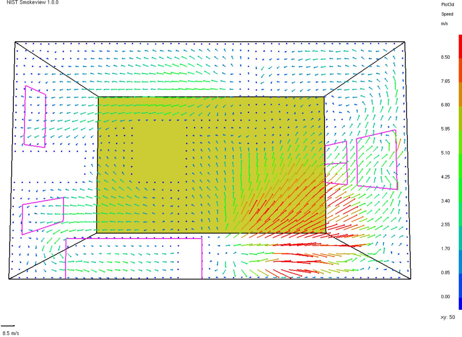
Figure 17. Vector representation of velocity at the ceiling with first floor sliding glass door vented, at 200 seconds of simulation.
