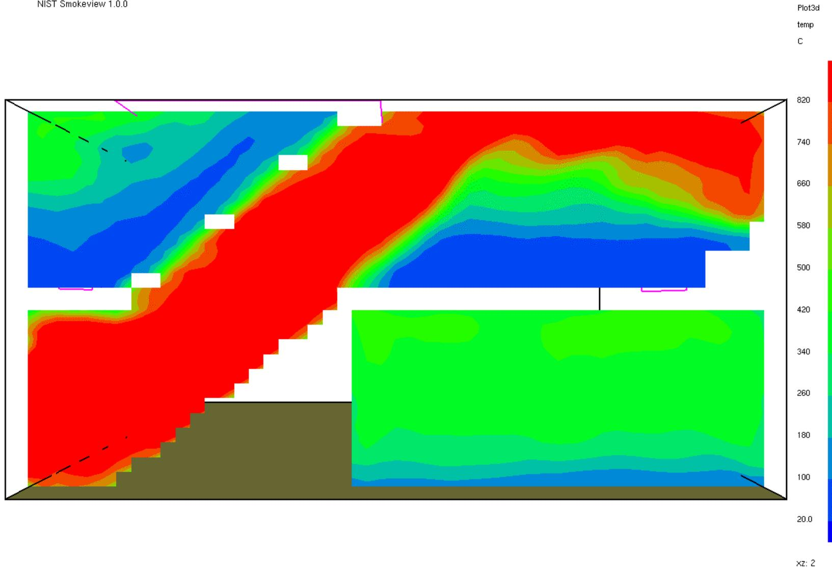
Figure 16. Temperature slice along center line of stairway with first floor sliding glass door vented, at 200 seconds of simulation.
