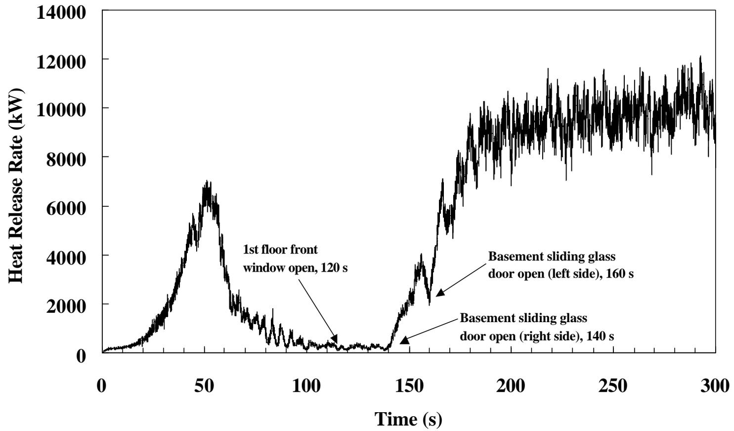
Figure 3. Heat release rate from FDS Simulation.
