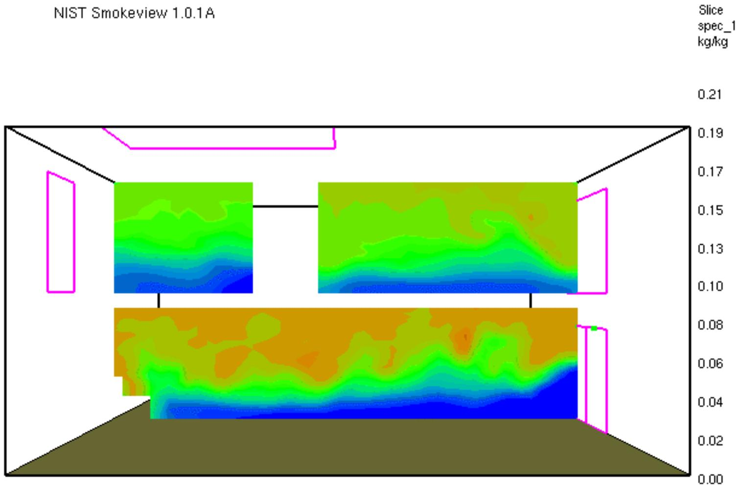
Figure 12. Percent oxygen along basement sliding glass door, at 200 seconds of simulation.
