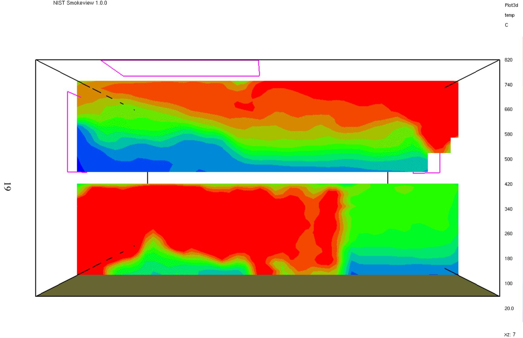
Figure 8. Temperature slice along front door, at 200 seconds of simulation.
